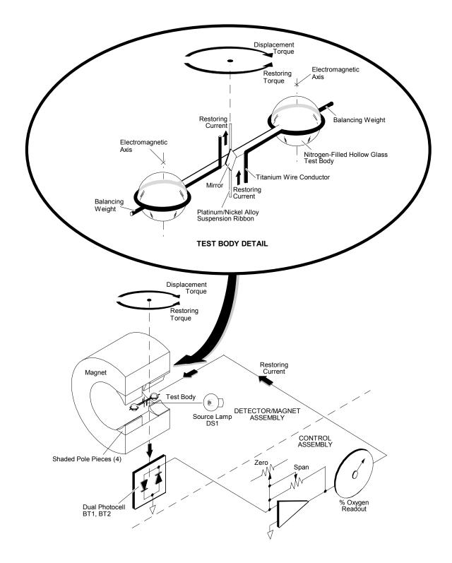
Figure 4-2. Functional Diagram of Model 755A Paramagnetic Oxygen Measurement System
